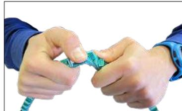
2. Flexing the belt as much as needed, twist and insert the second tab through the end link.
