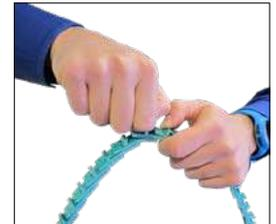
3. Ensure that tab will stay perpendicular to the belt's running direction; reverse the belt upside down to let it run on the tab side.
