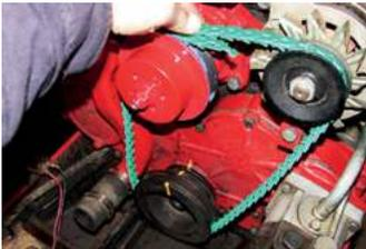
1. Pull the belt tight around the sheaves to check the needed length, overlap the last two tabs where two holes matching (as shown above).
