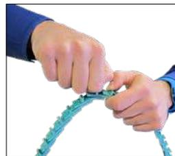
2. Twist one tab 90° to make it parallel to the belt; this way you can pull the end of the link over the tab.
