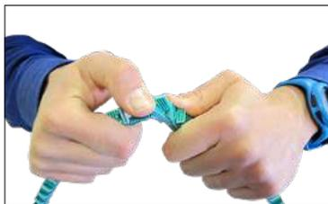
1. Put the belt with the tabs upwards and bend it as much as possible.
