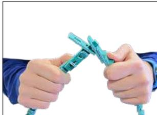
1. Holding the belt with the tabs upwards, let the tab of one belts' end go through two links (three if C section) at once.
