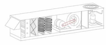
Rooftop Units (RTU) are air handlers designed for outdoor use, typically located on roofs. They are also known as packaged units (PU). The main difference is that they are usually more compact and because they are typically installed on the roof they need to be more robust and weather proof. While AHU's are often connected to a central plant such as chillers and boilers, RTU's are self contained and have everything all in one unit.
