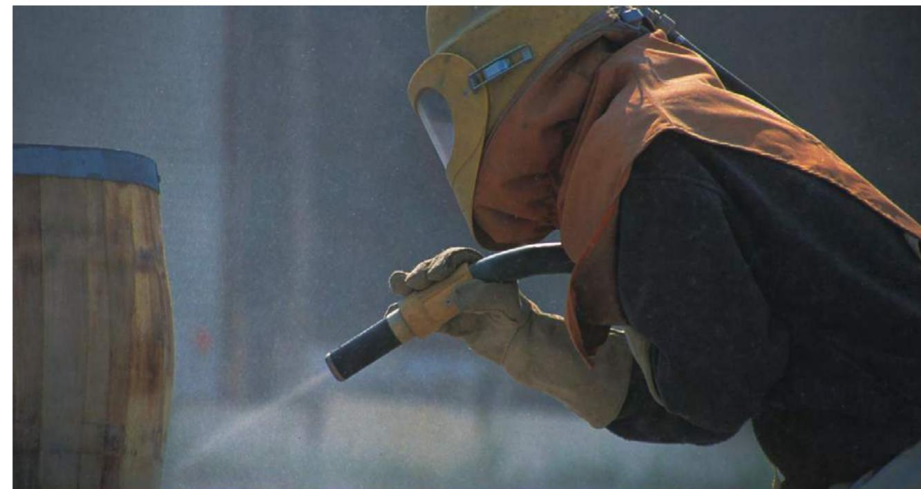
The flow of certain materials inside of a hose can cause a dangerous static charge to build up. When the static charge reaches a sufficient level, it can shock or create an electrical discharge which can lead to fire and explosions.
