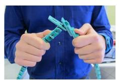
3. Flex belt further and insert second tab through end link by twisting tab with thumb.
