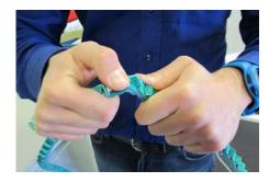
3. Rotate belt end with tab 90°.
