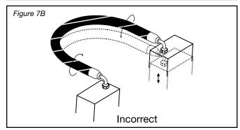
**5.24.2** – Prevent Hose Bending in More Than One Plane – if the hose follows a compound bend, couple it into separate segments that flex only in one place.
