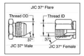
SAE J514 37° JIC Flare Thread Size and Maximum Working Pressure
