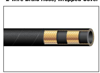
**APPLICATIONS:** Used for high pressure hydraulic lines on off-road construction equipment, machine tools, farm and marine equipment. Meets or exceeds SAE 100R2 and EN 853 2SN.
