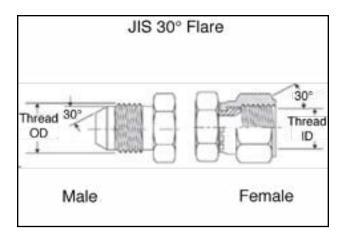
JIS 30° Flare with Parallel Pipe Threads Size
