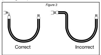
**5.23 - Lengths -** Unnecessarily long hose can increase pressure drop and affect system performance. When pressurized, hose that is too short may pull loose from its fittings, or stress the fitting connections, causing premature metallic or seal failures. When establishing hose length, refer to Figures 4, 5 and 6. Use the following practices:
