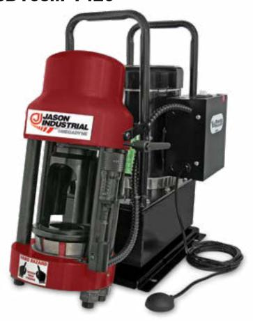
The JCD165M-T420 Series crimper with micrometer style adjustment and 62 tons of crimping force has the capability to crimp 4 spiral hoses up to 1-1/4".
