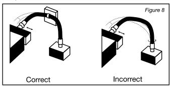
**6. Hose-Assembly Fabrication –** Persons fabricating hose assemblies should be trained in the proper use of equipment and materials. The
